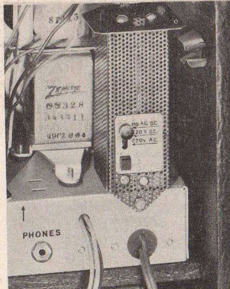
Figure 4.—Ballast Adaptor Inserted in Socket.
